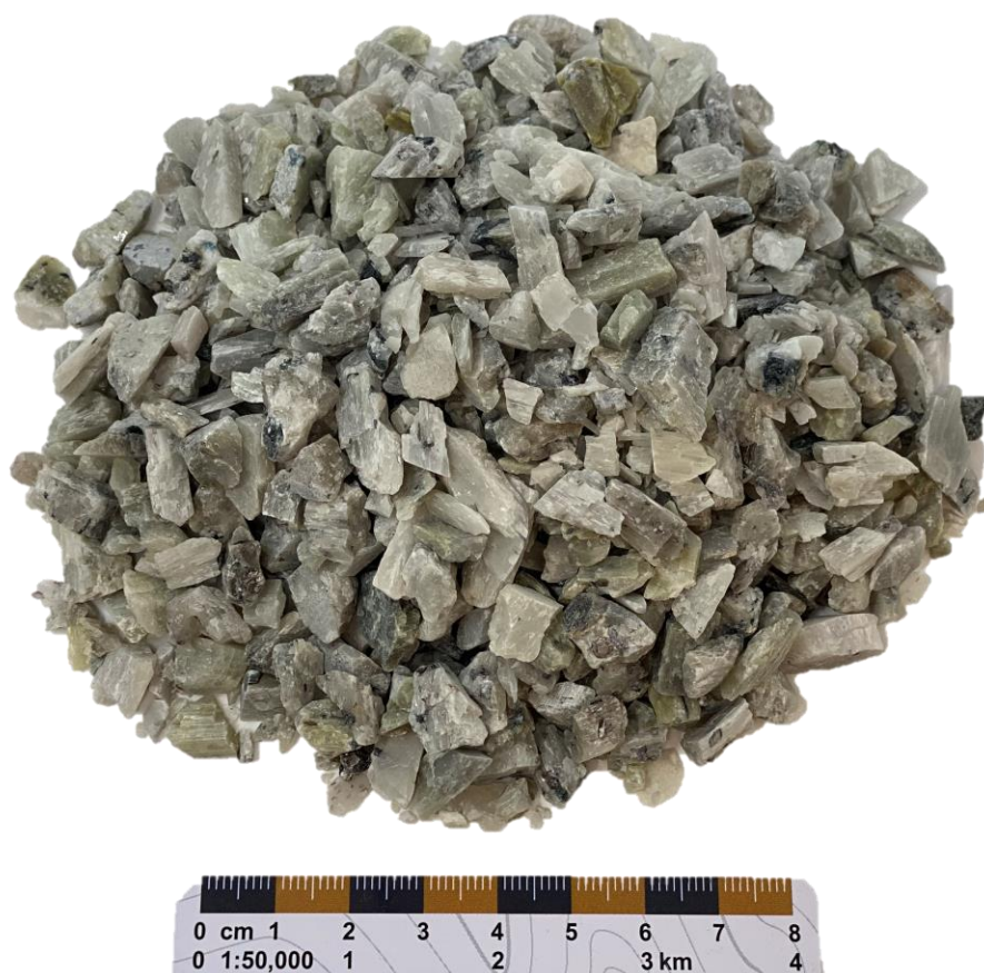
Figure 13-8: Spodumene concentrate (DMS + non-magnetic fractions) 5.8% \text{Li}_2\text{O} and 0.60% \text{Fe}_2\text{O}_3 at 79% recovery
