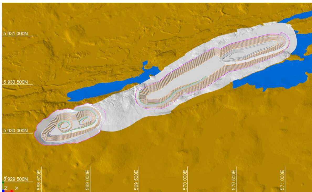
Figure 16-10: Phase 3 pit design
