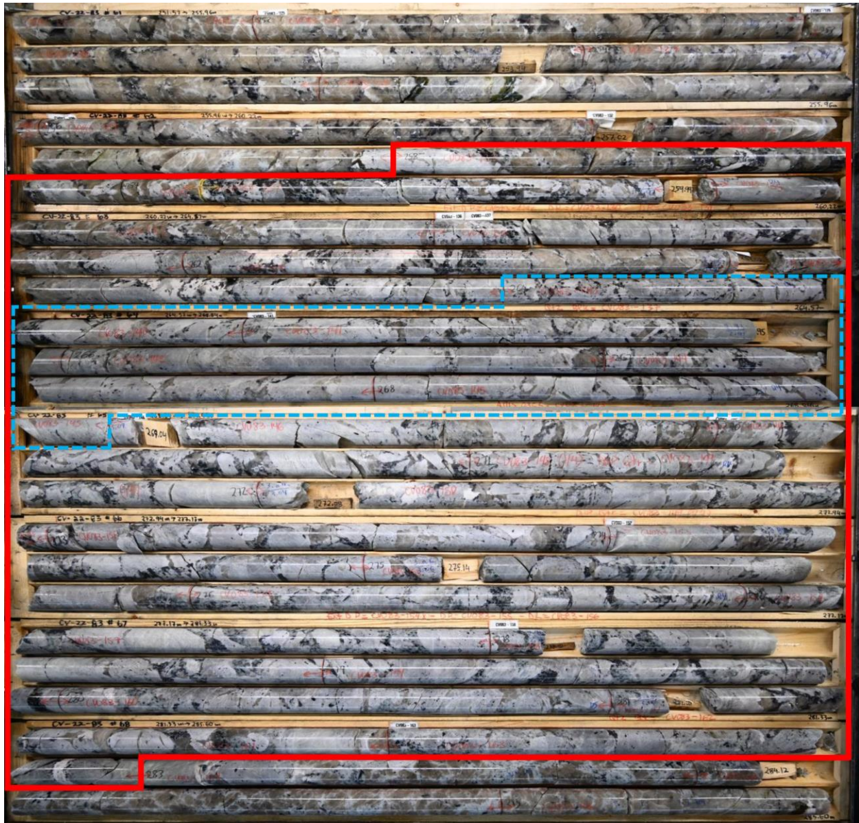
Figure 10-7: Nova Zone drill core intersection (25.0 m at 5.04% \text{Li}_2\text{O} ) in CV22-083 (red box) including 5.0 m at 6.36% \text{Li}_2\text{O} (dashed blue box)
