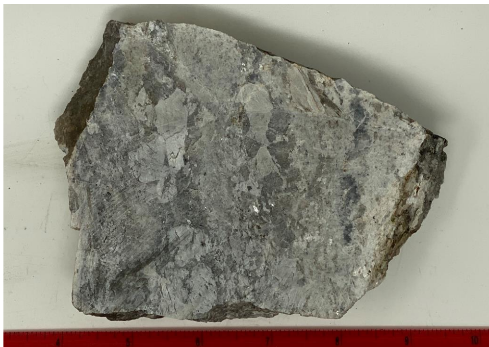
Figure 7-32: Spodumene crystals in saw-cut sample from CV10
