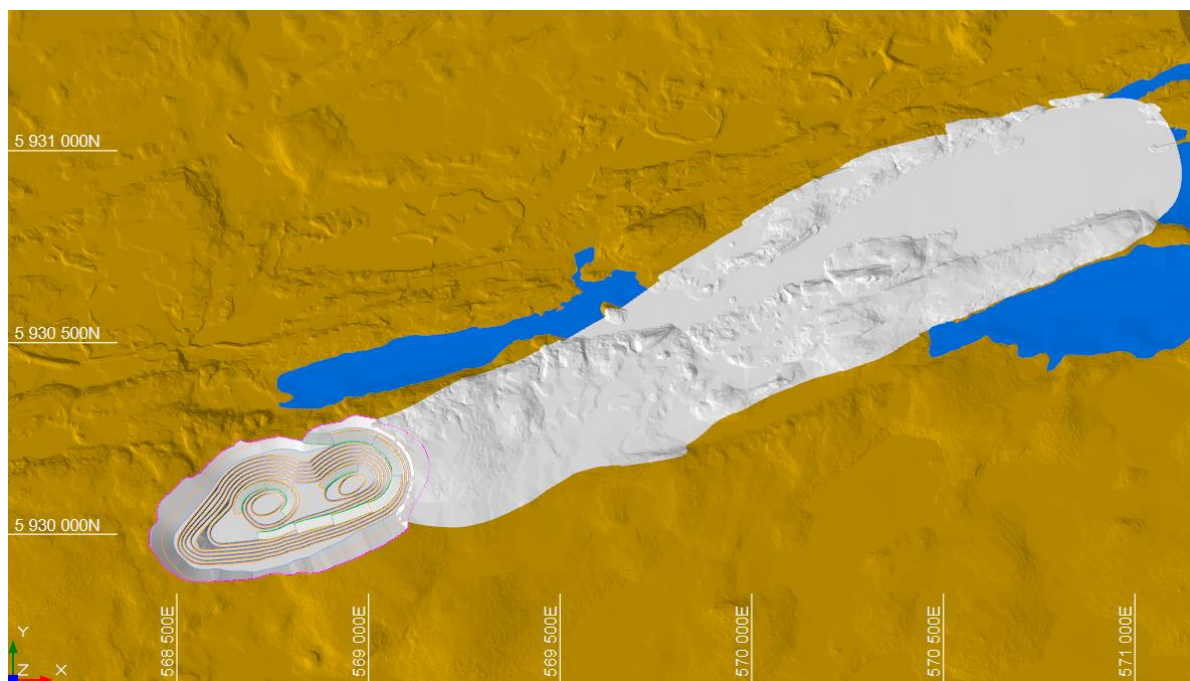
Figure 16-8: Phase 1 pit design
