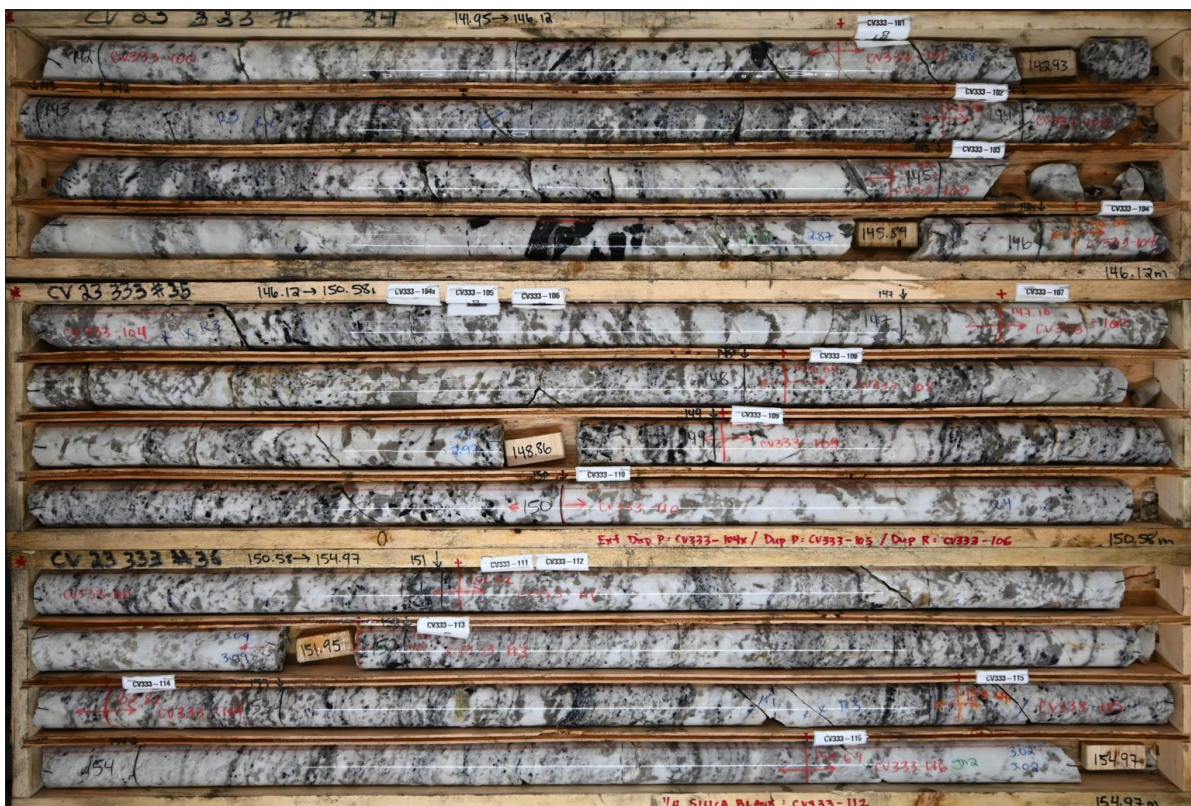
Figure 10-15: Spodumene pegmatite from drill hole CV23-333, including 7.7 m at 1.35% Li 2 O (146.0 m to 153.7 m)
