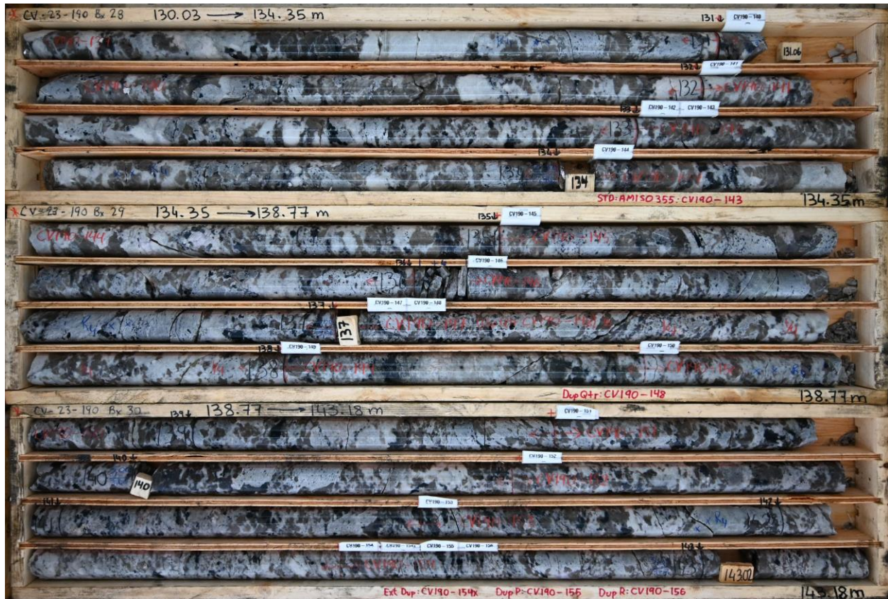
Figure 10-8: Spodumene pegmatite from drill hole CV23-190 grading ~1.8% Li 2 O
