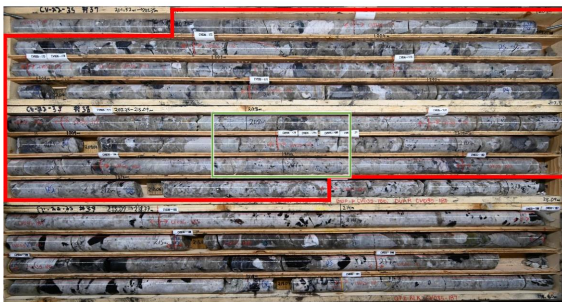
High-grade lithium mineralized drill intersection in CV22-035 – 3.29% \text{Li}_2\text{O} and 177 ppm \text{Ta}_2\text{O}_5 over 10.0 m (202.5 m to 212.5 m – red box) within a wider zone of 1.25% \text{Li}_2\text{O} and 118 ppm \text{Ta}_2\text{O}_5 over 96.9 m (126.1 m to 223.0 m)
