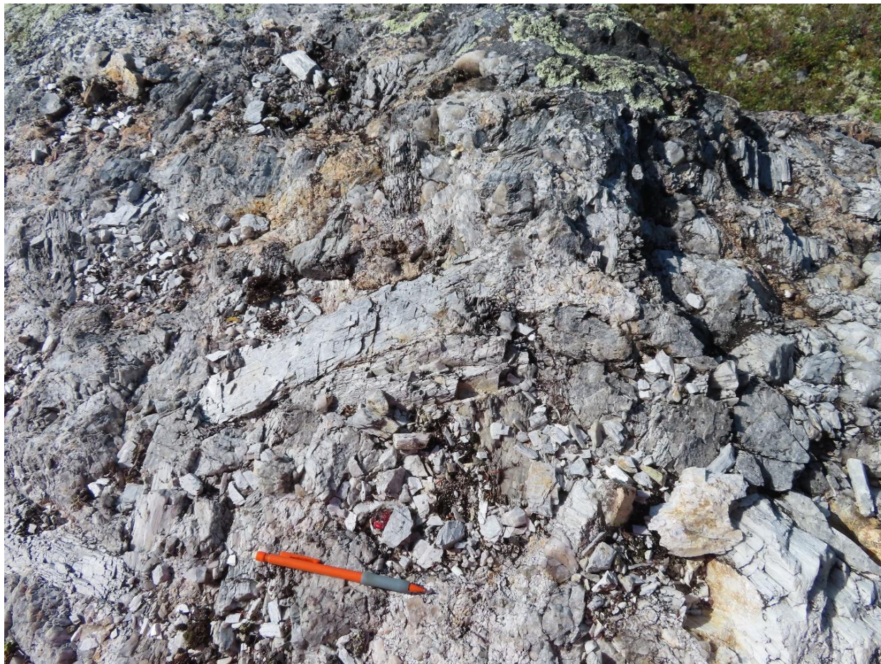
Figure 7-26: Very coarse, grey spodumene in the easternmost outcrop at CV8 (6.72% \text{Li}_2\text{O} , sample 124302)
