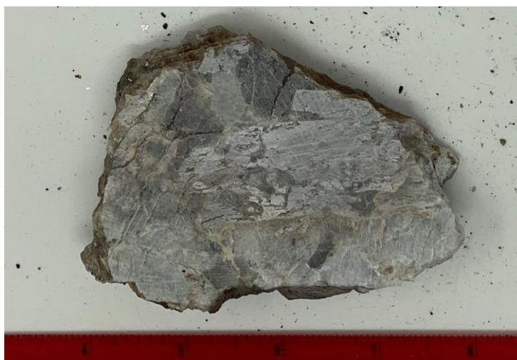
Figure 7-21: Coarse-grained spodumene crystals in saw-cut grab sample from CV13
