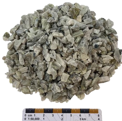
Figure 1-3: Final concentrate product generated from the CV5 Pegmatite via DMS
