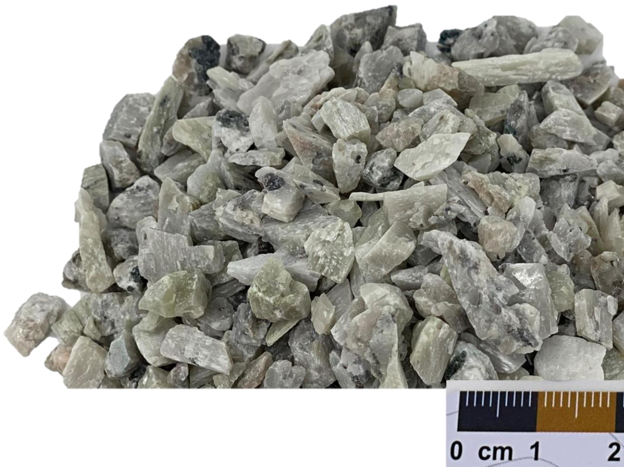
Figure 13-9: Close-up of spodumene concentrate (DMS + non-magnetic fractions) 5.8% \text{Li}_2\text{O} and 0.60% \text{Fe}_2\text{O}_3 at 79% recovery
