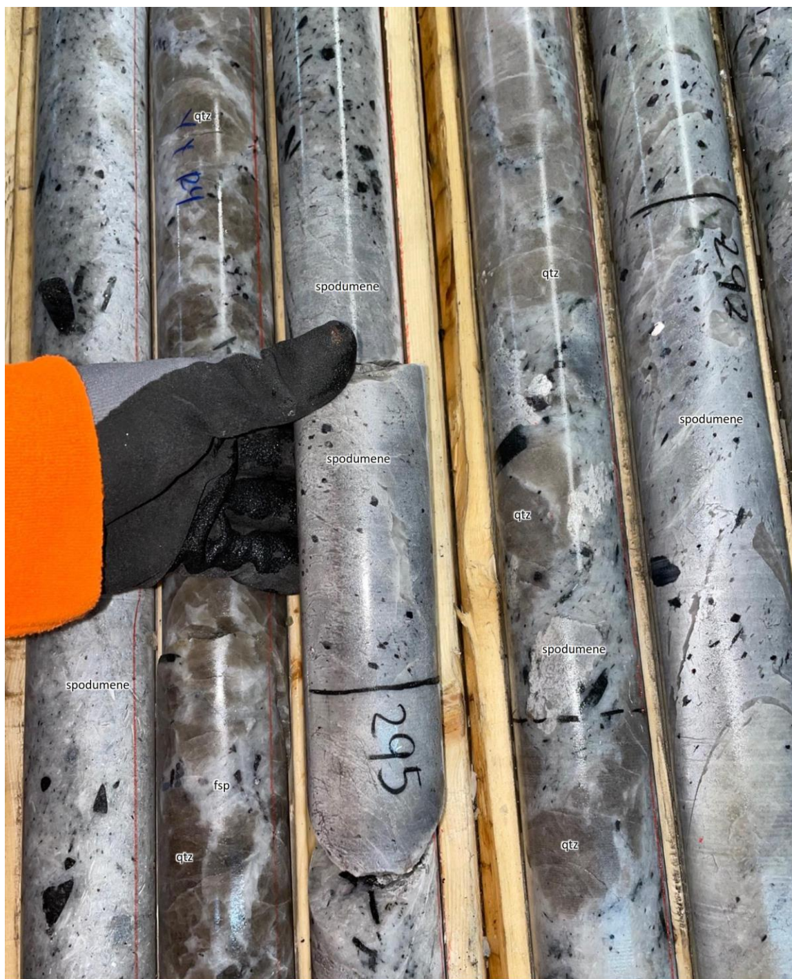
Figure 7-12: Coarse-grained spodumene mineralization in drill hole CV22-083
