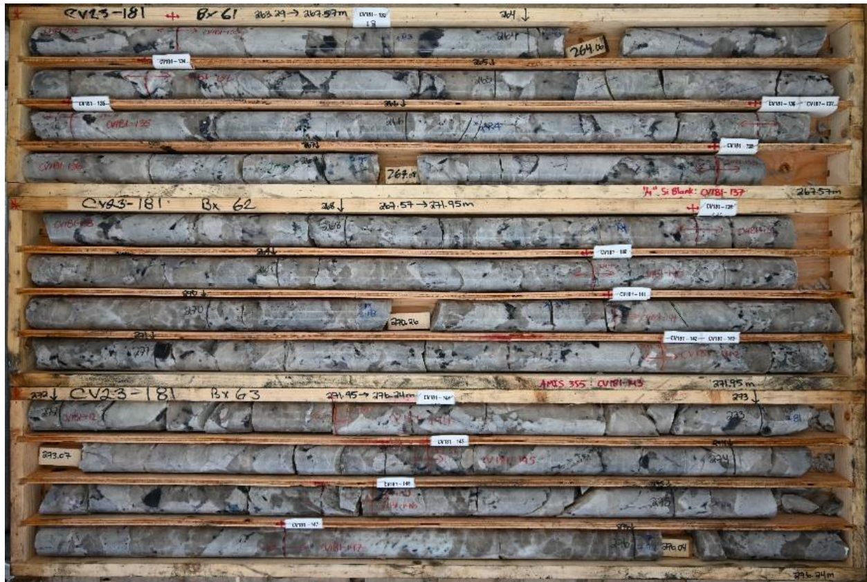
Figure 10-9: High-grade (4+% \text{Li}_2\text{O} ) spodumene pegmatite from the Nova Zone in drill hole CV23-181
