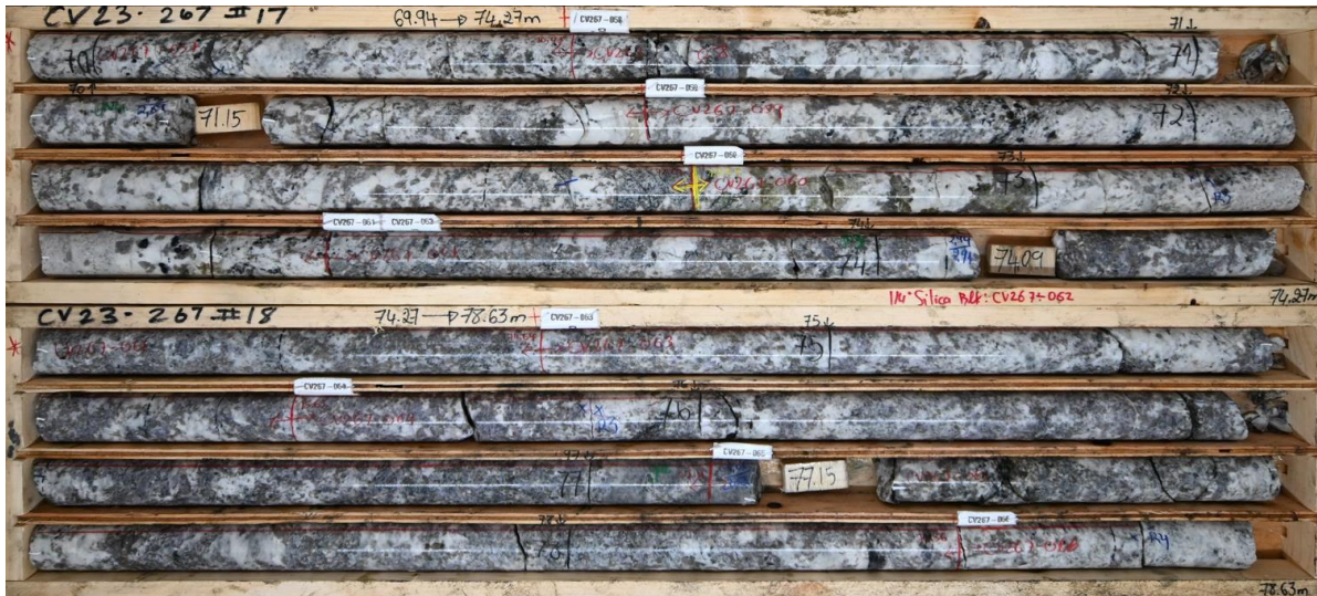
Figure 10-14: Spodumene pegmatite from drill hole CV23-267. Approx. 1.0% Li 2 O over interval (70.0 m to 78.6 m)
